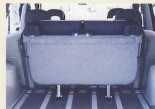
Rear view - seat folded forward. Folded seat takes up 300mm.
