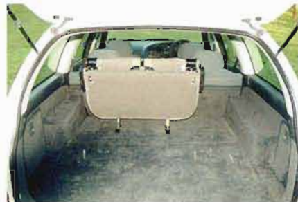
Rear View - showing seat folded forward for stowage.
